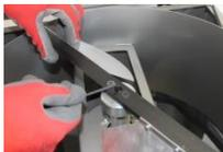
2 Loosen the central screw of the shaft.
