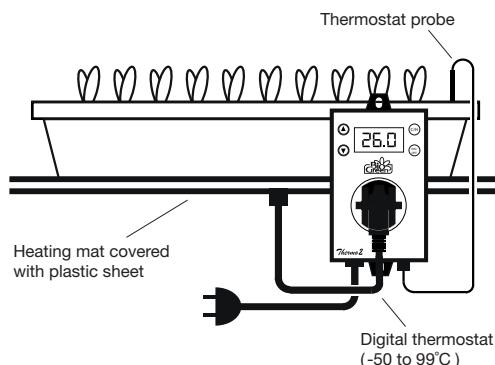
This saves energy, since the heat is generated near the roots. The heat supply is continuous and even, but not enough in most cases to prevent a sudden ambient temperature drop. A frost monitor is in addition required to do this.
